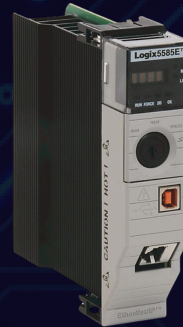
ControlLogix 5580: 1756 L81E Allen Bradley
